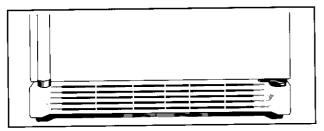
2. To level the refrigerator, use a screwdriver and turn roller adjusting screws clockwise to lower the cabinet or counterclockwise to raise the cabinet.
